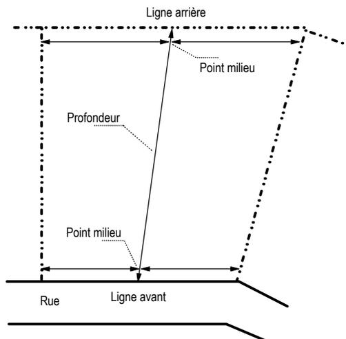
**FIGURE 5.1C : DIMENSIONS D'UN TERRAIN – LOT DE COIN**
