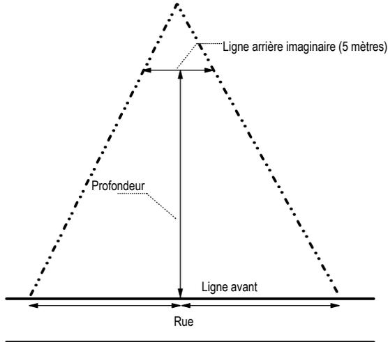
**FIGURE 5.1F : DIMENSIONS D'UN TERRAIN – IRRÉGULIER**
