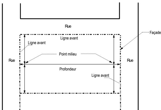
FIGURE 5.1B : DIMENSIONS D'UN TERRAIN – LOT INTÉRIEUR
