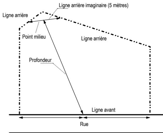
**FIGURE 5.1E : DIMENSIONS D'UN TERRAIN – IRRÉGULIER**
